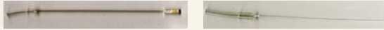
Figure 1 - Micro-glass cryostraw shown outside Cassou straw for freezing/thawing (right). The micro-glass cryostraws were inserted into Cassou straws (left) under liquid nitrogen for storage in tank.
